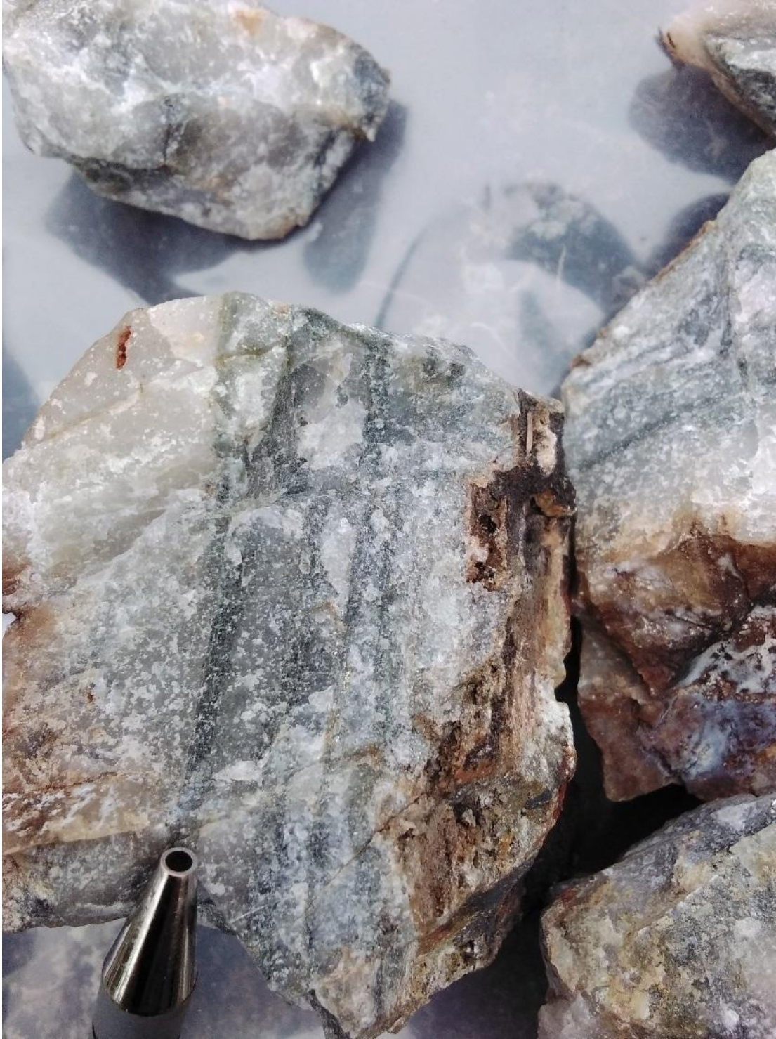
Photo 3 - 2021 New discovery gold-bearing vein. Shear plans of chlorite-bearing material within the quartz vein. Pyrite is also present within these plans, indicating it was affected by the deformation.
