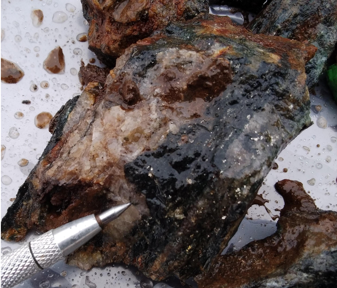
Photo 4 - 2021 new Georgekish discovery gold-bearing vein – 61.8 g/t Au and 35.8 g/t Ag in the north-central claim block of the Project. It consists of a deformed oxidized (from oxidation of sulphides) quartz vein hosted in chlorite-bearing altered conglomerates with disseminated pyrite.
