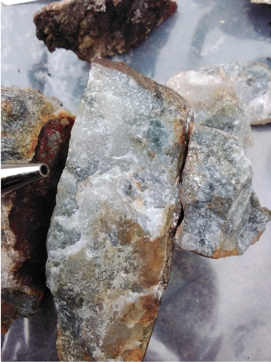
Photo 2 - Gold-bearing quartz vein with galena (lead-bearing), sphalerite (zinc-bearing), chalcopyrite (copper-bearing) and pyrite.
